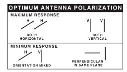
Figure 11: Antenna Polarization
