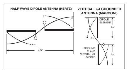
Figure 5: Dipole Antenna Operation
