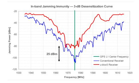
Figure 2: Measured directly at the GPS carrier frequency, an interference signal of only about –110 dBm is sufficient to degrade the signal by 3 dB for receivers using conventional approaches (red trace), whereas u-blox 5 / 6 can handle interference that is 25 dBm stronger before it reaches its 3-dB desensitization point (blue trace).
