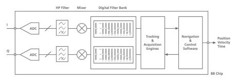
Figure 1: This simplified block diagram of a GPS receiver based on the u-blox 5 / 6 technology shows the SAW filter at the signal input to block out-of-band interference plus the softwarecontrolled digital filter bank that blanks out specific interference sources.
