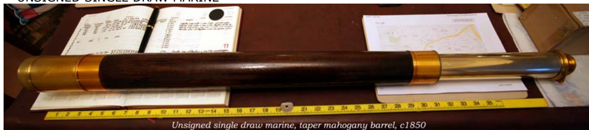
Unsigned single draw marine, taper mahogany barrel, barrel length 26&1/2", extended 45&1/4", Schyrle-Huyghens 4-lens eyepiece, x22.
