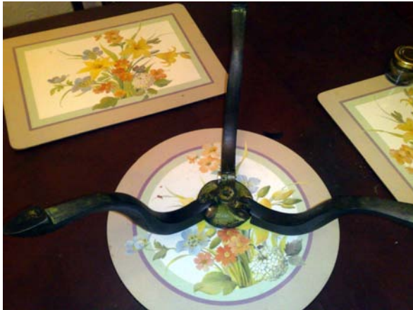
Husbands - claw legs - inverted & hinge boss - note centre punch marks used to assemble each leg & hinge pin correctly. Note also traces of lead chromate primer applied before the bronze gilding which had been rubbed off. New brass hinge pins were turned to suit, blackened with Selenium compound, and the cabriolé legs and hinge boss re-primed with lead chromate and gilded dark bronze.
