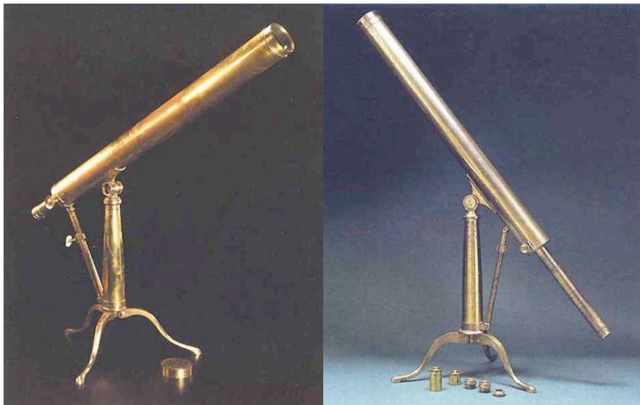
Ramsden, late C18th & Matthew Berge, London, early C19th - pillar & claw with pad feet & altitude adjustment. Matthew Berge apprenticed to Jesse Ramsden, his father or uncle, John Berge apprenticed to Peter Dollond.
