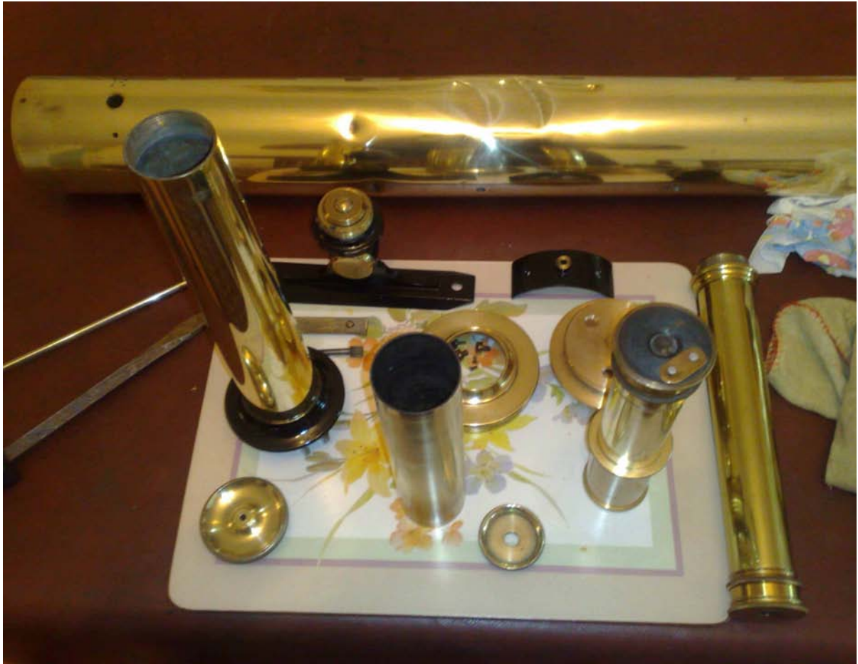
3-inch f/12 unsigned achromatic refractor, dismantled and re-polished using the technique described in the article (see restoring & maintaining antique & vintage brass refractors). In order from top: the brass barrel, heavily dented; altaz trunnion; pinion saddle plate; rack & pinion; racktube flange; tripod pillar cap; tripod pillar (prior to filling with lead shot); racktube; drawtube & eyecap; pinion wheel; altaz tensioning collar; B.C. & Co., Ltd., Pancratic eyepiece.
