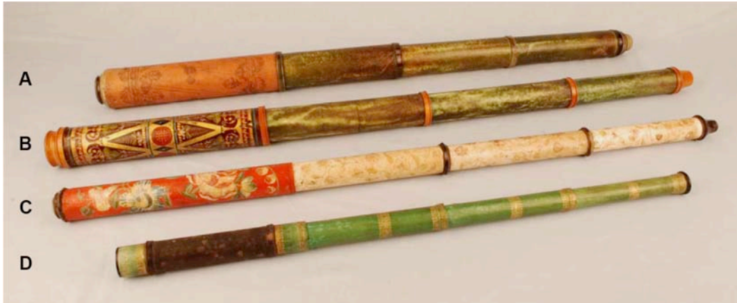
Pasteboard telescopes from the early to mid C18th: (A) Paper covered pasteboard barrel and vellum covered draws, fittings made of horn. Length 33", barrel dia. 2\frac{1}{4} " (Leonardo Semitecolo, Venice) (B) Painted tin covered barrel and vellum covered draws, fittings made of wood. Length 31\frac{7}{8} ", barrel dia. 1\frac{7}{8} " (unsigned German) (C) Painted paper covered pasteboard barrel and vellum covered draws, fittings made of horn. Length 32\frac{1}{4} ", barrel dia. 1\frac{5}{12} " (unsigned Italian) (D) Leather covered pasteboard barrel and vellum covered draws, fittings made of horn. Length 24\frac{13}{32} ", barrel dia. 1\frac{3}{16} " (unsigned French) Ref: Proc. of SPIE Vol. 8129 812902-5 Fig.5
