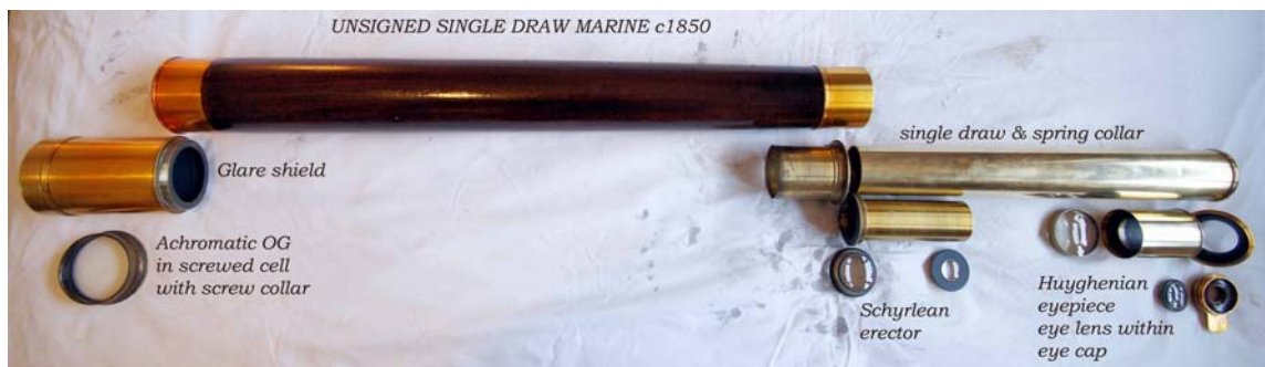
Unsigned single draw marine, taper mahogany barrel, barrel length 26&1/2", extended 45&1/4", Schyrle-Huyghens 4-lens eyepiece, x22.
