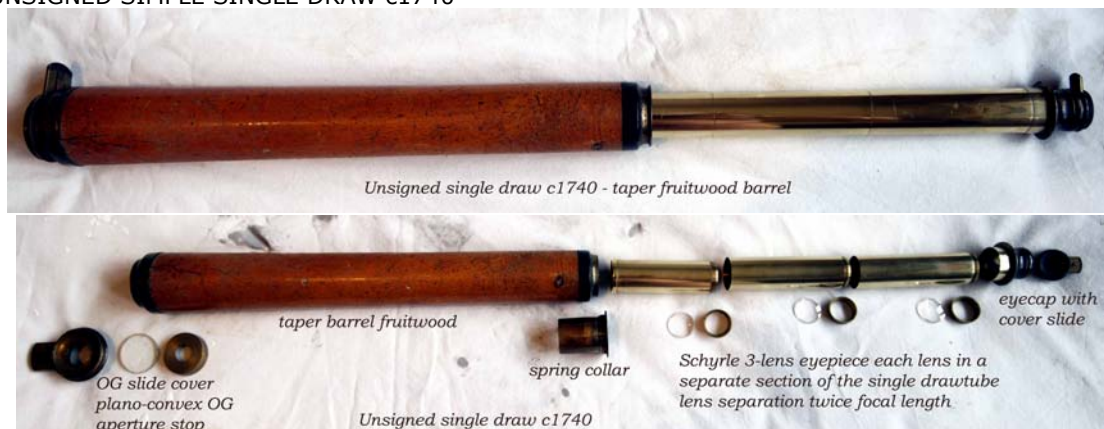
Single-draw pre-achromatic telescope with a taper fruitwood barrel and a Schyrle erecting system (unsigned c1740, English). The telescope has an barrel length 13&1/4", extended 21". The objective dia. 1".082 stopped down to 0".45.
