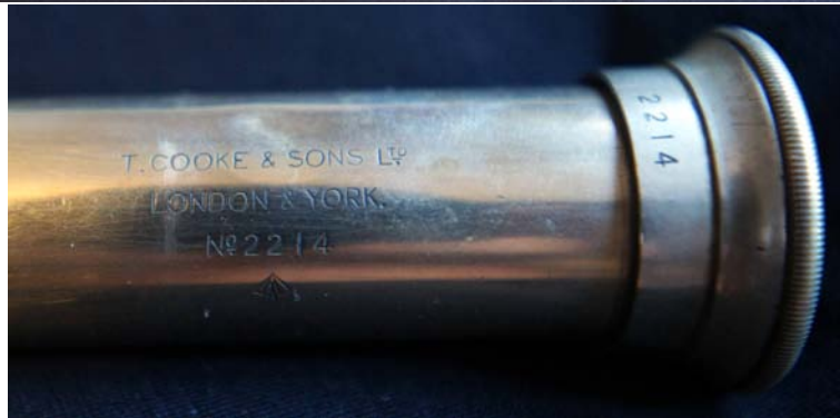
'Officer of the Watch' telescope, T. Cooke & Sons Ltd., London & York No.2214 c1915. Single-draw air-spaced contact achromatic telescope leather bound barrel and a Pancratic erecting system. The telescope has an barrel length 17 \frac{3}{8} " , extended 24 \frac{7}{8} ". The objective dia. 1 \frac{1}{4} ". Nickel plated brass. Magnification x10.
