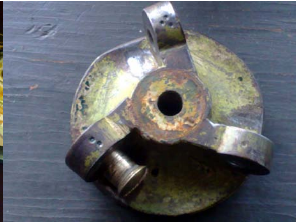
Husbands - claw legs - inverted & hinge boss - note centre punch marks used to assemble each leg & hinge pin correctly. Note also traces of lead chromate primer applied before the bronze gilding which had been rubbed off. New brass hinge pins were turned to suit, blackened with Selenium compound, and the cabriolé legs and hinge boss re-primed with lead chromate and gilded dark bronze.
