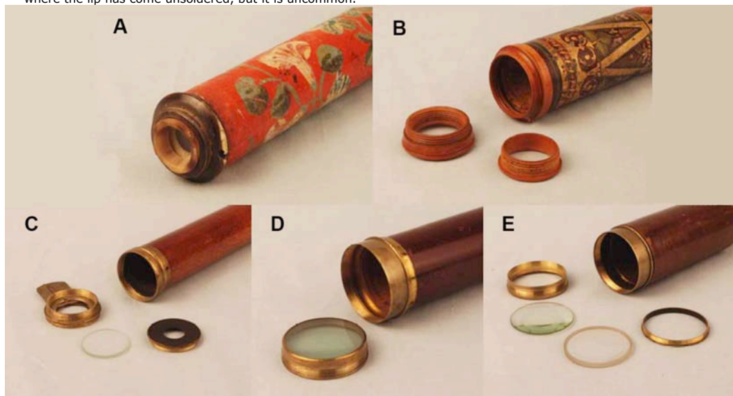
Objective lens mounting: (A) Lens is mounted in a turned horn cell with a retaining ring. The retaining ring is on the front of the lens cell. (Leonardo Semitecolo, Venice, early - mid C18th) (B) Lens is mounted in a turned wood cell with a wood retaining ring that screws into the rear of the cell (unsigned, German, early-mid C18th) (C) Brass cell with an integral dust slide in front. The lens is held in place by a cap with a built-in aperture stop. (unsigned, mid C18th, English) (D) Lenses are sealed together in a brass cell with a spun-over edge. (Dollond, London, c1800) (E) Lenses are mounted in a brass cell with a retaining ring. (Thomas Harris & Son, London, mid C19th.) Ref: Proc. of SPIE Vol. 8129 812909-3 Fig.8
