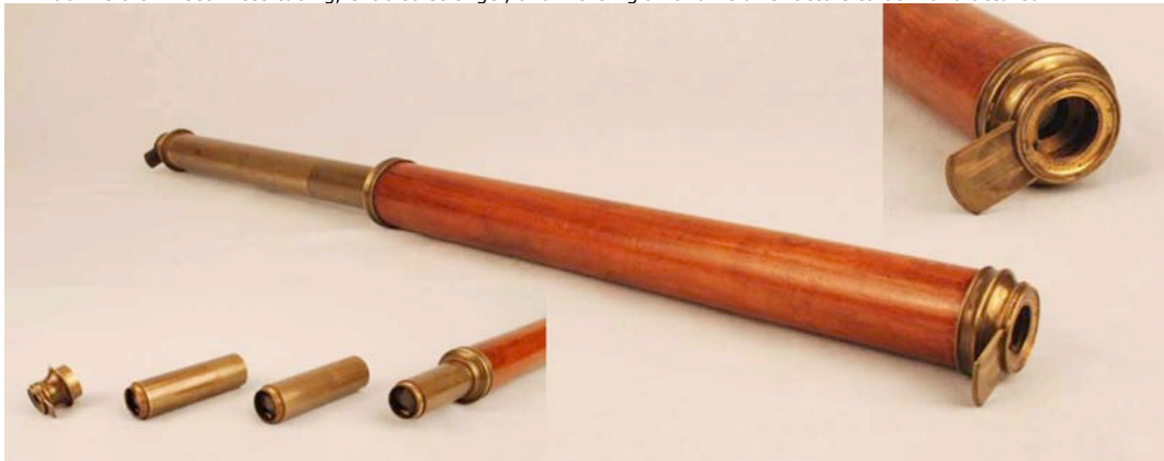
Single-draw pre-achromatic telescope with a wooden barrel and a Schyrle erecting system (unsigned c1740, English). The telescope has an overall length of 22\frac{7}{16} ". The objective dia. 1\frac{10}{128} " stopped down to 1\frac{31}{256} ". Each segment of the draw contains one of the three lenses of the Schyrle erecting system. Ref: Proc. of SPIE Vol. 8129 812902-4 Fig.3
