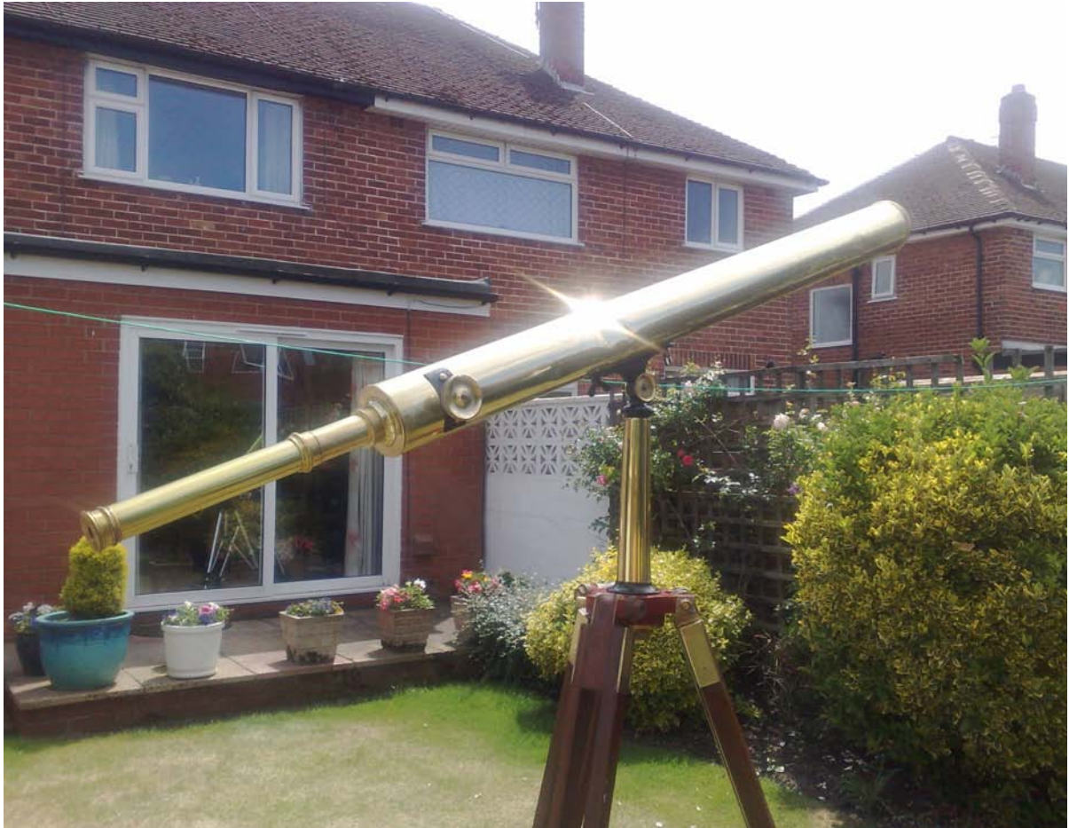
3-inch f/12 unsigned achromatic refractor, intended for both terrestrial and astronomical use. The barrel is red brass (62-38) c1880, and has 'season cracking'. The eyepiece is a Broadhurst, Clarkson & Co., Ltd., Pancratic c1910, RAS screw fitting. The original object glass which would have been very similar to a spare B.C. & Co., Ltd., 3" f/13 achromatic doublet in my collection, dating from the 1910's, has been replaced with a Conrady design achromatic triplet c1960.
