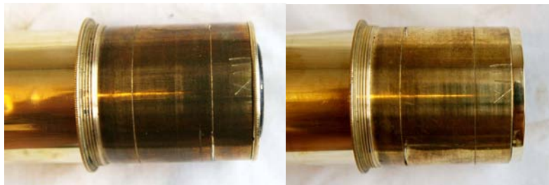
brass jobber's assembly marks on spring collars
