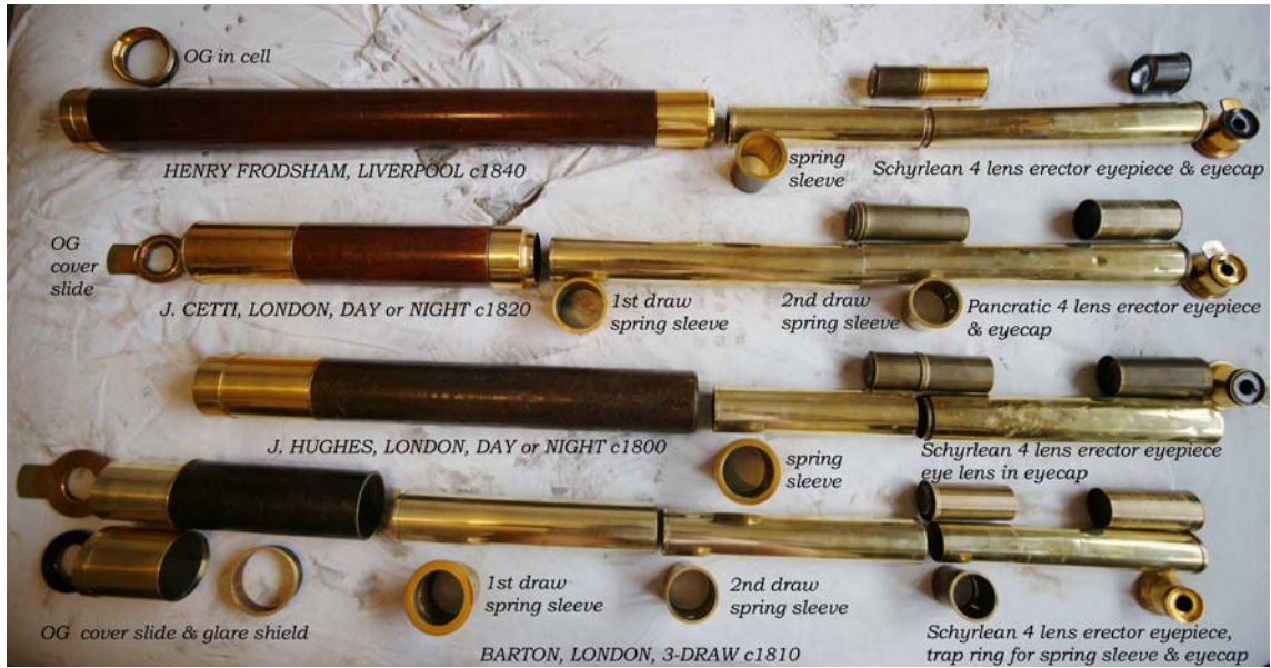
Frodsham - OG dia. 1.815/16" x 28"fl - split drawtube with Schyrle 4 lens eyepiece (original eyepiece missing) J. Cetti - OG dia. 1.81/2" x 31.81/4"fl - 2 draw, Pancratic 4 lens eyepiece within 2nd draw. J. Hughes - OG dia 1.81/2" x 17"fl - split drawtube with Schyrle 4 lens eyepiece. Barton - OG dia. 1.81/4" missing - 3 draw with Schyrle 4 lens eyepiece within third draw.
