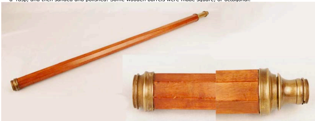
Reverse taper octagonal telescope (unsigned c1750, English). The length of the telescope is 42\frac{117}{128} ", the barrel dia. 1\frac{3}{10} " at the objective end widening to 1\frac{21}{32} " at the eyepiece end. Ref: Proc. of SPIE Vol. 8129 812902-5 Fig.4
