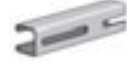
AS 500S Channel w/ Long Slots Size: 1 1/2" x 1 3/8" x 14 GA. 1 1/2" x 3" Slots on 4" Centers Page 33
