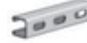
AS 520EH Channel w/ Elongated Holes Size: 1 1/2" x 1 3/8" x 12 GA. 3/8" x 1 1/8" Elongated Holes on 2" Centers Page 34
