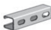
AS 210EH SS/ZD/HG Channel w/ Elongated Holes Size: 1 1/2" x 1 1/2" x 14 GA. 3/8" x 1 1/8" Elongated Holes on 2" Centers Page 87
