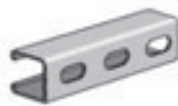
AS 200EH SS/ZD/HG Channel w/ Elongated Holes Size: 1 1/2" x 1 1/2" x 12 GA. 3/8" x 1 1/8" Elongated Holes on 2" Centers Page 86
