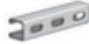
AS 400EH Channel w/ Elongated Holes Size: 1 1/2" x 1" x 12 GA. 3/8" x 1 1/8" Elongated Holes on 2" Centers Page 32
