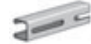
AS 400S Channel w/ Long Slots Size: 1 1/2" x 1" x 12 GA. 1 1/2" x 3" Slots on 4" Centers Page 32
