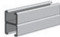
AS 200BTB EH SS/ZD/HG Welded Channel Size: 1 1/2" x 3 1/2" x 12 GA. Two Pcs. AS 200EH Welded Back-to-Back 3/8" x 1 1/8" Elongated Holes on 2" Centers Page 86
