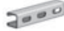
AS 500EH Channel w/ Elongated Holes Size: 1 1/2" x 1 3/8" x 14 GA. 3/8" x 1 1/8" Elongated Holes on 2" Centers Page 33
