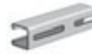
AS 300S Channel w/ Long Slots Size: 1 1/2" x 1 1/2" x 12 GA. 1 1/2" x 3" Slots on 4" Centers Page 31
