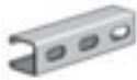
AS 300EH Channel w/ Elongated Holes Size: 1 1/2" x 1 1/2" x 12 GA. 3/8" x 1 1/8" Elongated Holes on 2" Centers Page 31
