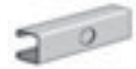
AS 400KO Channel w/ Knock Outs Size: 1 1/2" x 1" x 12 GA. 7/8" Knock Outs on 6" Centers Page 32
