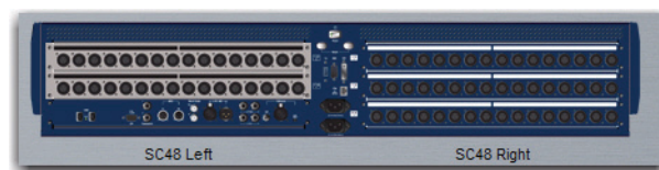
Detail of Devices tab indicating presence of two A016 Cards output slots D and E
