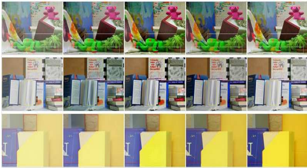
Figure 5. Visual results on dehazing synthetic images. From left to right columns: hazy images, DehazeNet results [3], MSCNN results [17], AOD-Net results, and the groundtruth images. Please amplify to view the detail differences in bounded regions.
