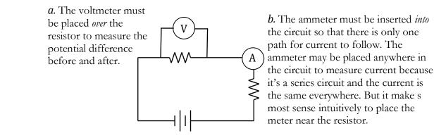
1. The two resistors are in series, so the current I is the same throughout the circuit. Using Ohm's Law and the information we have for  $R_1$ :
