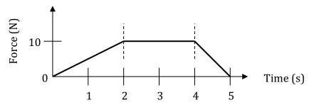
An object of mass m = 2.0kg experiences a force in Newtons according to the *Force* vs. *time* graph shown here. For the time interval shown, what is the total change in momentum of the object?
