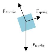
b. The force of gravity acting down the ramp ( $F_{g-parallel}$ ) pulls down on the mass until the force of the spring is pushing up with an equal amount of force. (See diagram next page.)
