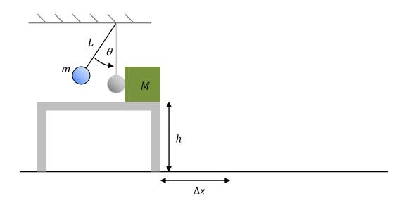
A pendulum of length L = 1.0 meter and bob with mass m = 1.0 kg is released from rest at an angle  $\theta = 30^{\circ}$  from the vertical. When the pendulum reaches the vertical position, the bob strikes a mass M = 3.0 kg that is resting on a frictionless table that has a height b = 0.85m.
