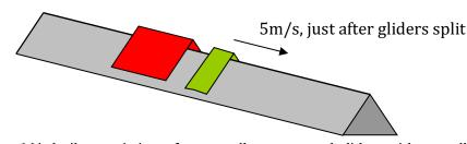
An air track glider of mass M is built, consisting of two smaller connected gliders with a small explosive charge located between them. The glider is traveling along a frictionless rail at 2 m/s to the right when the charge is detonated, causing the smaller glider with mass  $\frac{1}{4}M$ , to move off to the right at 5 m/s. What is the final velocity of the second small glider?
