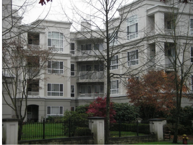
Figure 5.3.7 - Planning for access to building perimeter is essential if boom lifts are to be used. Capacity of parking garage roof slab and hard and soft landscaping features are critical considerations.
