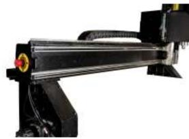
**Gantry Custom Engineered for Maximum Rigidity**Made of 3/8" thick steel tube, the gantry is welded, stress
