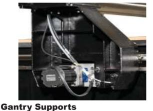
**High Strength, Minimal Vibration**In conjunction with wide X-axis bearing spacing, cast-iron gantry supports help dampen vibration and give the structural tube gantry extremely rigid support.
