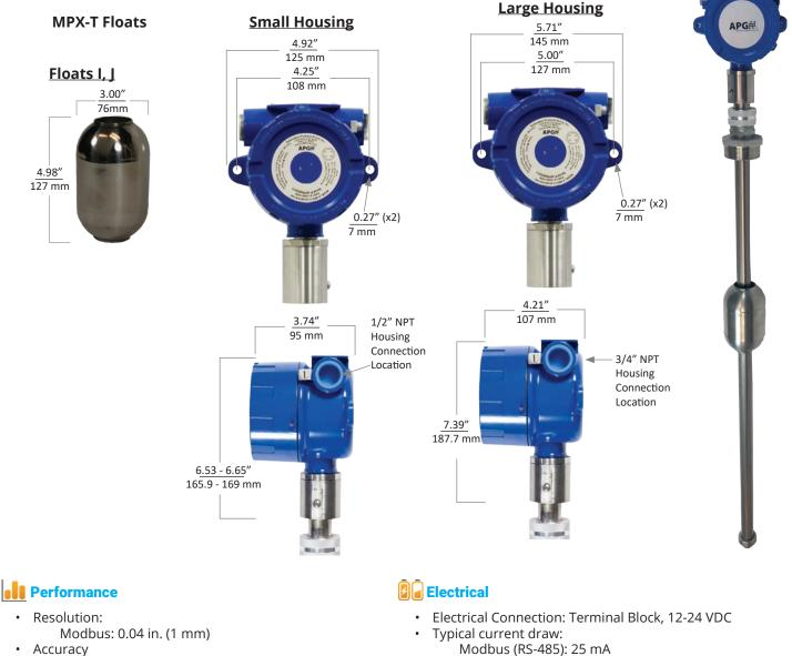
±0.04 in. (1 mm) over range Distance: Temp Sensors: ±0.25°C over -40° - 85°C ±0.13°C over +20° - 70°C
