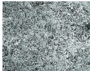
Figure 2: Acceptable microstructure after welding (100X)
