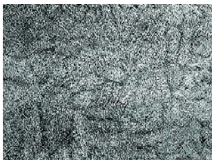
Figure 1: Acceptable microstructure after casting (100X)
