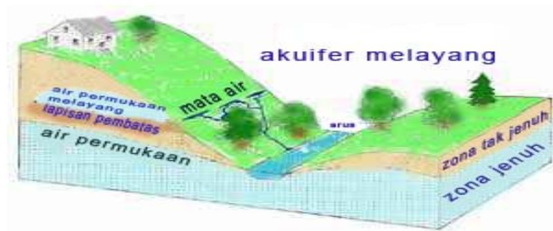
Gambar 2.5 Akuifer melayang ( Perched Aquifer )
