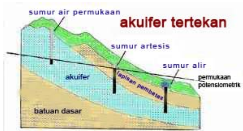
Gambar 2.3 Akuifer tertekan ( Confined Aquifer )
