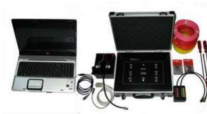
Gambar 3.2 Alat resistivitas S-Field 16 elektroda otomatis multichannel
