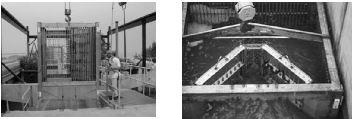
Figure 1. Fish trapping baskets were re-designed in 2000 to more effectively sample fish entering Metzger Marsh. Photo on left shows the grate system used to limit access by larger fish and the crane used to lift the basket from the water. Photo on right shows the entrance to the basket guarded by "fingers" to prevent escape once fish have entered the trap
