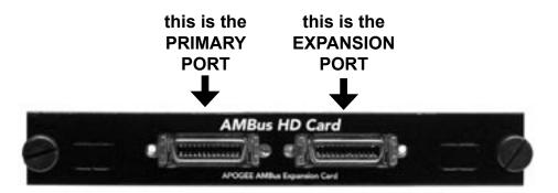
The proper order to connect Apogee, Digidesign and Prism hardware interfaces may be determined by locating the entry on pages 13-14 that corresponds to the set of interfaces you wish to connect. *When using Digidesign or Prism interfaces, please note that they must be connected first in the Digilink chain.*
