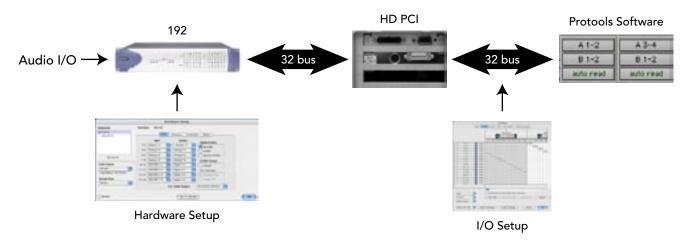
As the audio I/O of Apogee interfaces differs from that of a 192 I/O, a connected Apogee interface will ignore all settings in the Hardware Setup which pertain to audio I/O on the hardware. To define how audio I/O on an Apogee interface is routed to the 32 I/O busses (through the AMBus HD card), settings should be configured from the unit's front panel.
