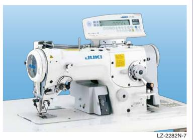
High-speed, 1-needle, Lockstitch, Zigzag Stitching Machine
