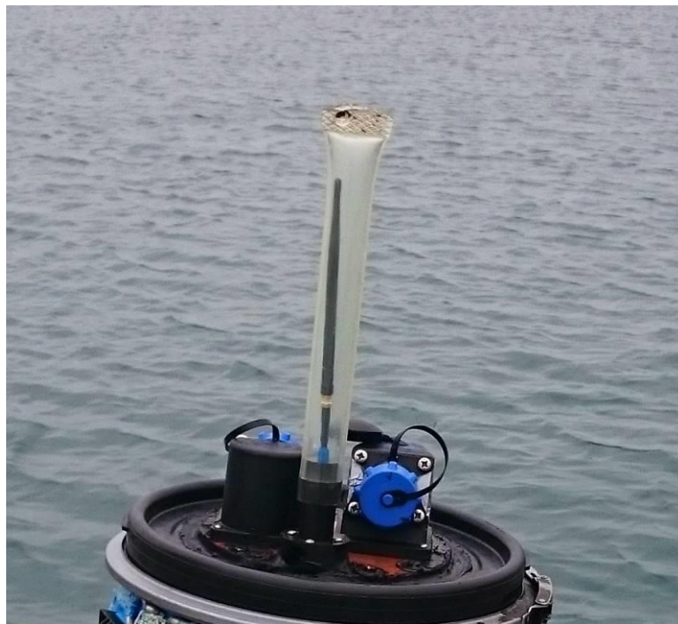
Figure 9. Custom enclosure for Wi-Fi aerial consisting of specially turned plastic base and a length of sealed polyurethanes tube
