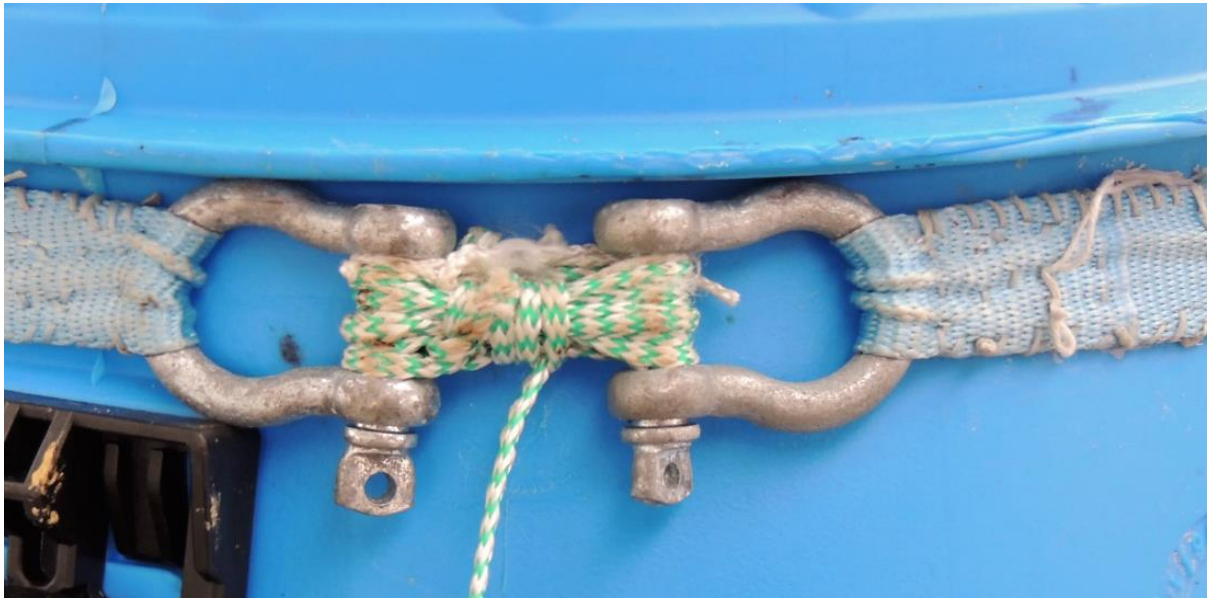
Figure 4 Shackles and lashing used to tension the cross straps
