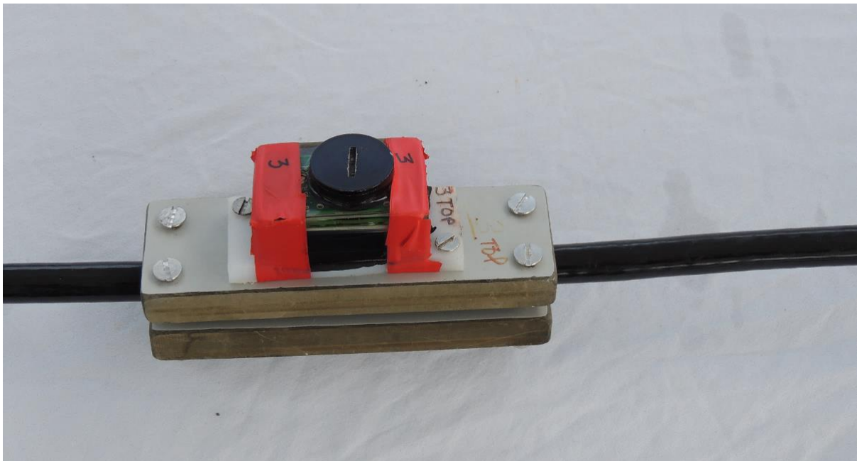
Figure 20 Mount for Open Tag on the cable of the vertical array.
