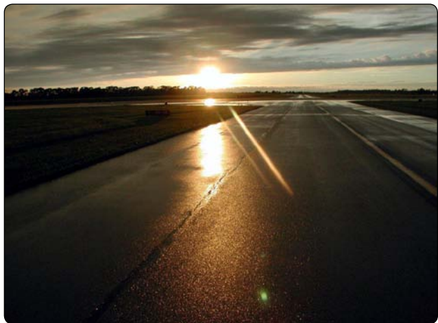
Figure 1-9. Low sun angle is obscuring the runway holding position sign and marking at a taxiway/runway intersection.
