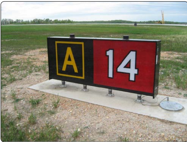
Figure 1-19. Runway holding position sign at takeoff end of Runway 14 with collocated Taxiway Alpha location sign.
