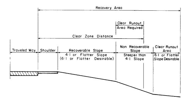
FIGURE A-2-4 EXAMPLE OF A PARALLEL EMBANKMENT SLOPE DESIGN
