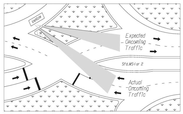
FIGURE A-3-7 DIAGRAM OF EXPECTED ONCOMING TRAFFIC VERSUS ACTUAL ONCOMING TRAFFIC
