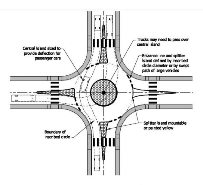
Features of a Typical Mini-Roundabout\*
