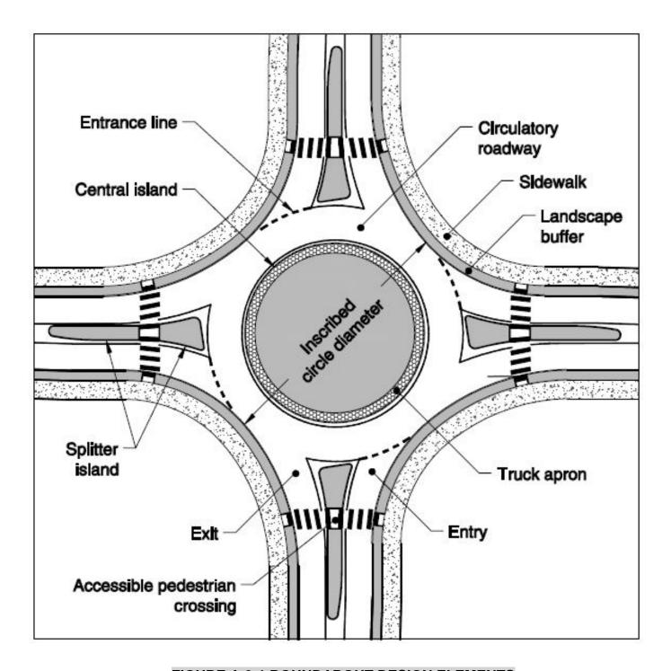
FIGURE A-3-1 ROUNDABOUT DESIGN ELEMENTS
