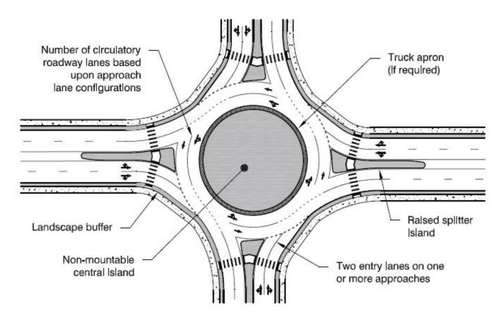
Features of a Typical Multi-Lane Roundabout
