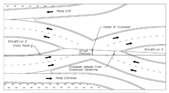
FIGURE A-3-5 OFFSET DISTANCE FOR INTERSECTION
