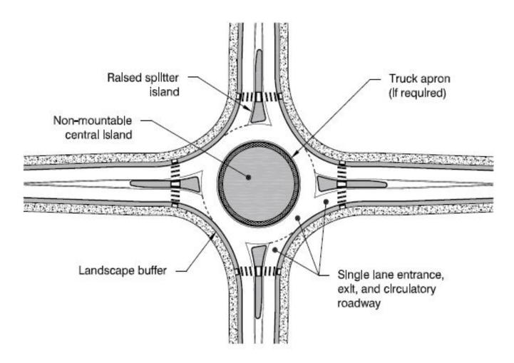
Features of a Typical Single-Lane Roundabout
