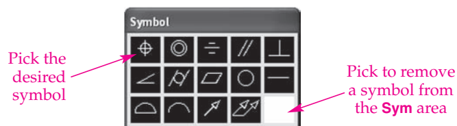
Figure A1-2. Use the Symbol dialog box to select a geometric characteristic symbol for use in a feature control frame.
