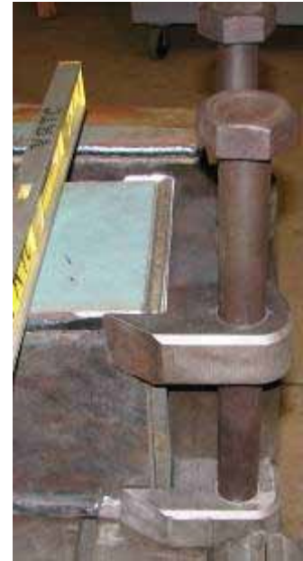
Figure 4.3: Left: Base Plate is added to the end. Middle: Base plate is welded to the Outboard Beam in the locations that the Hinge Brackets will overlap. Right: Hinge Brackets are being jigged up to weld. The bolts shown in the photo were removed and a aluminum jig was inserted into the holes to assure alignment, see Figure 4.4 (Middle).
