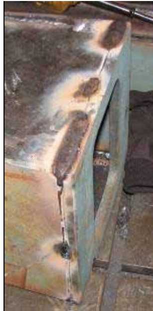
Figure 4.3: Left: Base Plate is added to the end. Middle: Base plate is welded to the Outboard Beam in the locations that the Hinge Brackets will overlap. Right: Hinge Brackets are being jigged up to weld. The bolts shown in the photo were removed and a aluminum jig was inserted into the holes to assure alignment, see Figure 4.4 (Middle).
