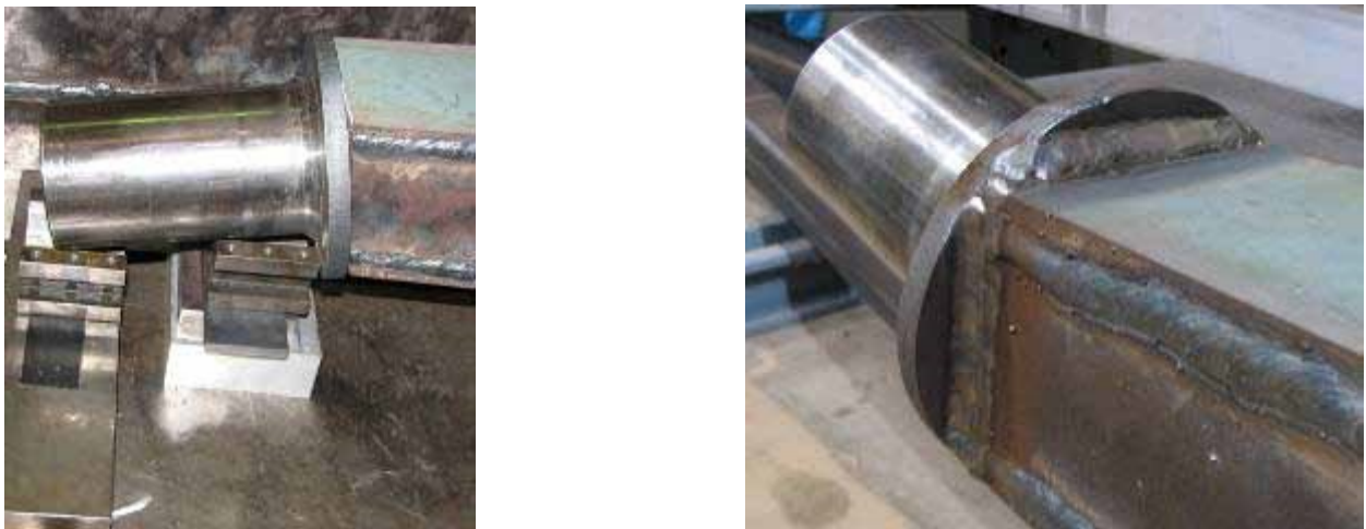
Figure 4.6: Left: End Plate and Axle Shaft are jigged into place for final attachment to the Outboard Beam of the new outriggers. Right: All seams are welded, multiple weld passes maybe necessary. Outboard Beam is complete.
