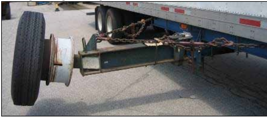
Figure 3.3: Photo of the UMTRI outrigger truck wheel/tire axle assembly; it uses a dual wheel with one tire mounted on the outer rim.
