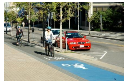
Curb Protected Sidewalk Level
