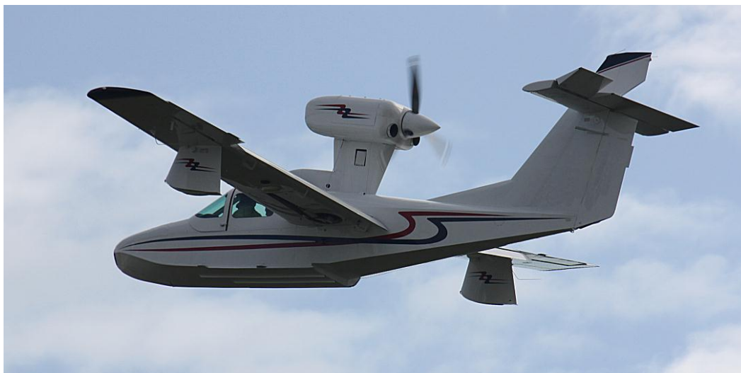
Figure C3-1: A Lake LA-250 Renegade, shown here during climb after T-O, is a popular option for amphibious aircraft. The large deflected flap on the horizontal tail is a hydraulically actuated trim tab used for slow speed operations only. It trims out the thrust effect of the highly mounted piston-propeller, improving its handling. (Photo by Phil Rademacher)
