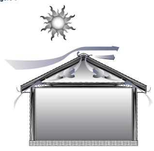
Thermal Flow (effect whereby cooler air falls, warmer air rises) and Natural Flow (effect due to wind) come together to ventilate an attic.
