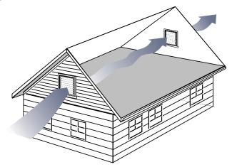
With wind blowing parallel to the ridge, airflow dips towards the attic floor leaving the hottest air still on the underside of the roof sheathing.
