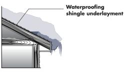
(Top) Water can penetrate to an unprotected roof sheath causing the roof sheath to rot.
