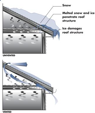
Unvented: Heat entering attic from the home melts the snow on the roof and forms destructive ice dams.
