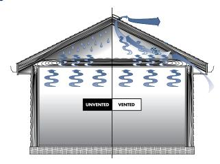
Unvented: Moisture rising up through the house condenses in the attic, causing damage to studs, insulation, and other materials. Vented: A vented attic allows moisture to escape.
