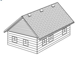
A roof louver is an exhaust vent located near the ridge.
