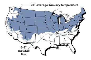
Above the 6-8" snowline concern should be given to the prevention of ice dams forming on the eave of the roof.
