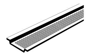
Continuous soffit vent takes in outside air and is located on the underside of the eave.
