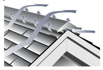
A baffled ridge vent creates an area of low pressure on both sides of the ridge vent. It literally pulls air out of the attic.
