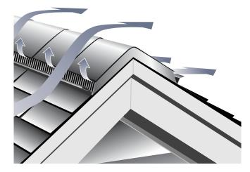
An externally baffled vent "pulls" air from the attic from both sides of the ridge vent.
