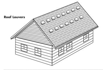
Fifteen roof louvers are required to equal the exhaust venting of 42 linear feet of ridge vent. This clearly demonstrates the performance and aesthetic advantages of ridge vents.
