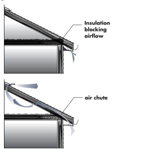
(Top) Insulation blocks undereave intake vents preventing proper airflow into the attic.
