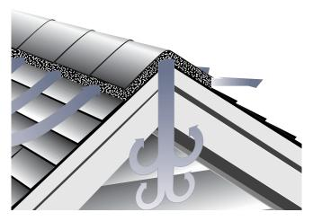
A roll vent with an internal baffle, or without any baffle at all, does not "pull" air from the attic.
