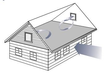
With wind blowing perpendicular to the ridge, the louvers act as both intake and exhaust vents.
