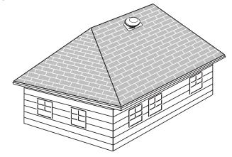
Power fans are used to move large volumes of air – a good option for hard-to-vent hip roofs that have limited horizontal ridge length available for ridge venting.
