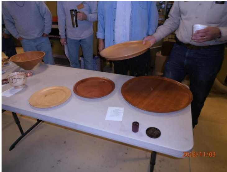
Tom Boley - 4 trays (cherry, ash, rosewood & maple), salad bowl oil finish, produced with double-sided tape method
