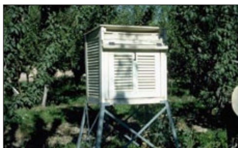
Weather monitors such as this help to calculate growing degree days. Photo: Howard F. Schwartz, Bugwood.org
