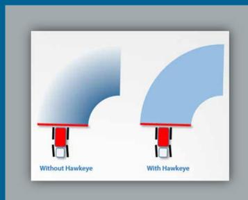
The Hawkeye® Nozzle Control System uses turn compensation to minimize over and under applications.
