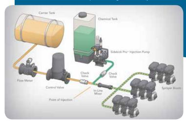
It's the direct injection system that sets a new standard for chemical applications of every type, with unprecedented precision, savings and safety. No tank mixing required —and with the industry's first remote and closed calibration and prime feature, you're ready to go in minutes. It also features:
