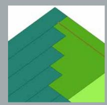
Examples shown are simulated on a 1 foot machine with 7 sections, 16 virtu sections, and 72 Hawkeye HD individu nozzle control. The field had a boundar without point rows and the sprayer exit the field at a 45 degree angle to the field boundary.
