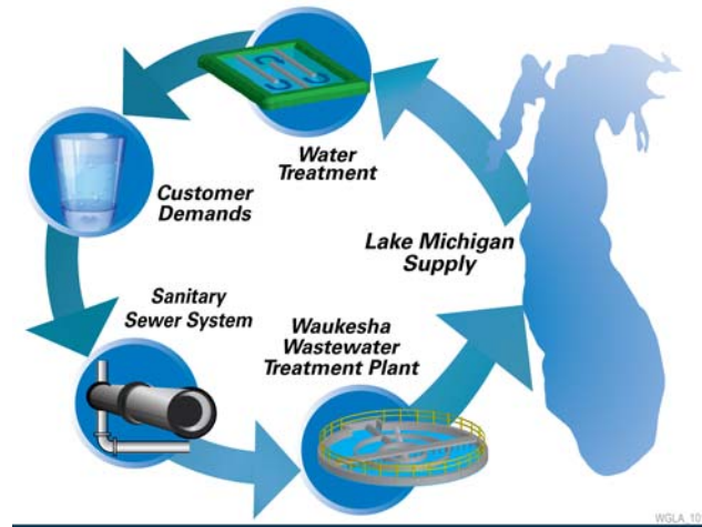
EXHIBIT 1-2 Proposed Supply, Treatment, and Discharge System
