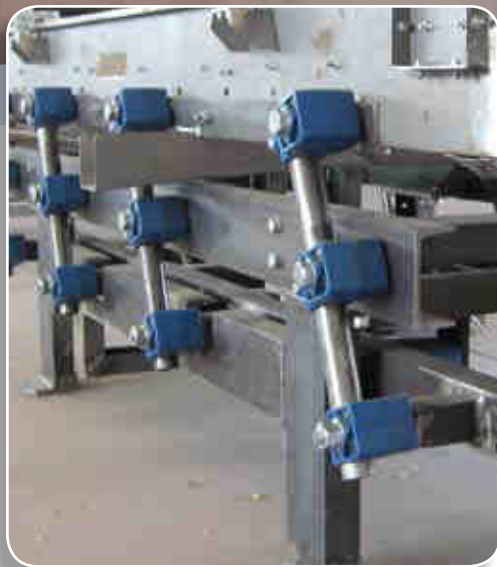
Fully adjustable double rockers for mass balanced systems
