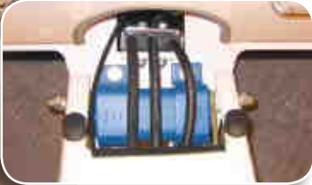
◀ Resilient handle mounting for vibrating compactors
