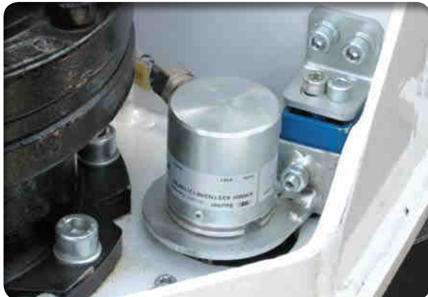
Elastic torque bracket for hydraulic motor
