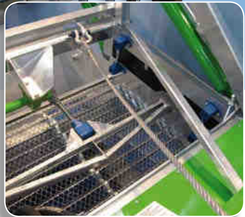
Elastic rocker suspensions for sand sifting screens
