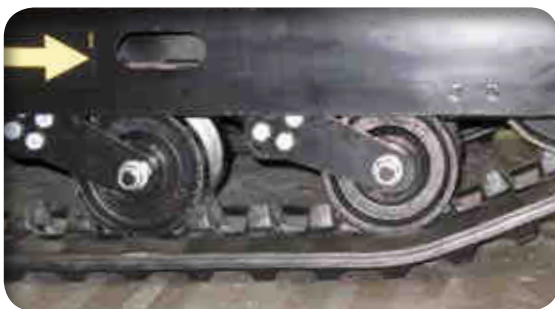
Elastic guide-wheel suspension for crawler mounted vehicles
