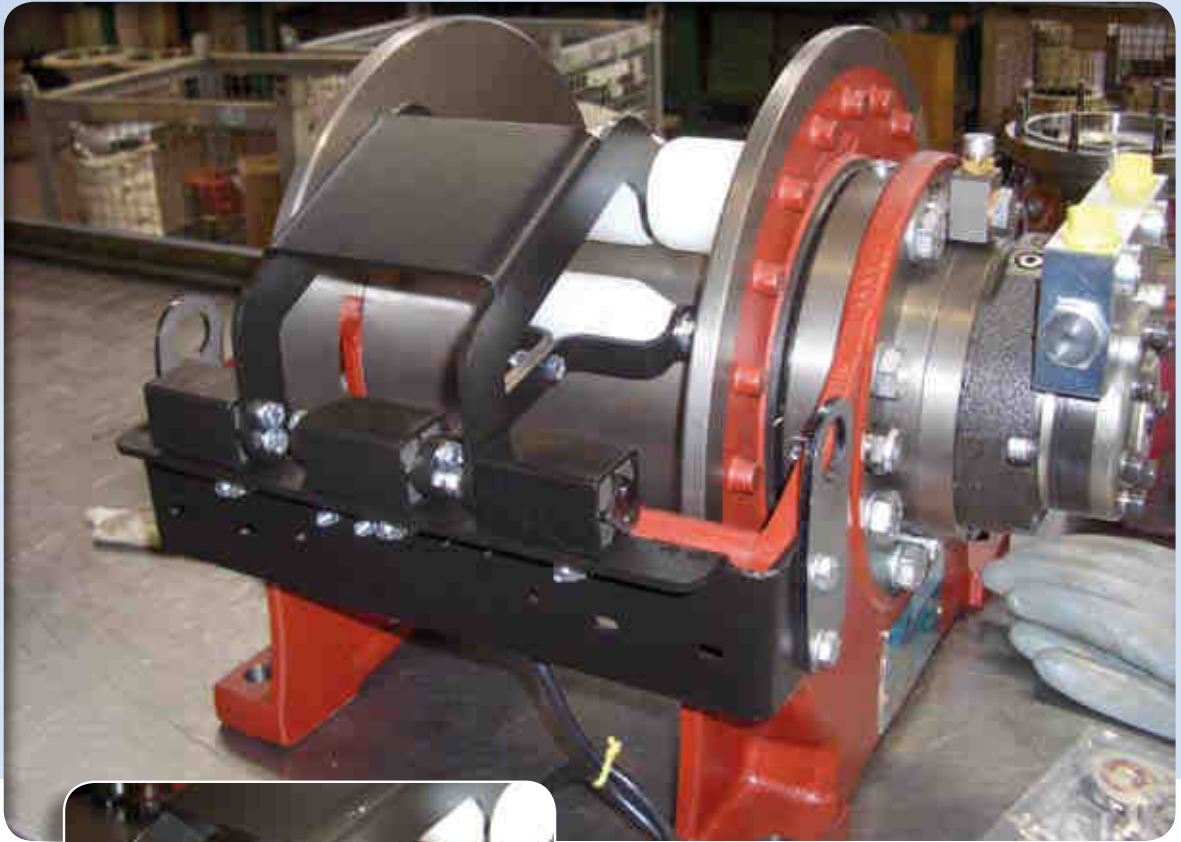
Guide roller suspensions for controlled cable reeling on winch drum
