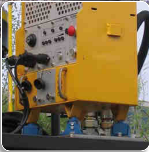
▲ Protective suspension of electronic device on track car
