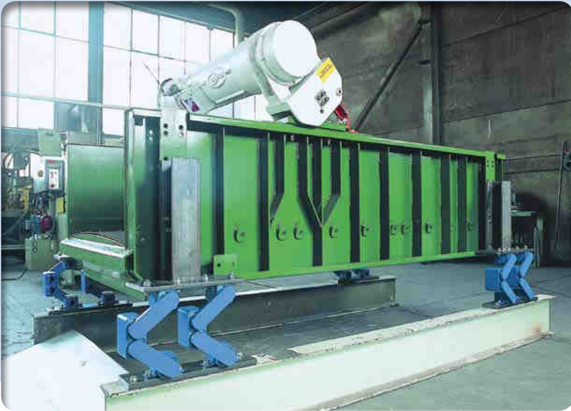
Elastic pendulum-suspension of single vibrators generating an ellipsoidal motion
