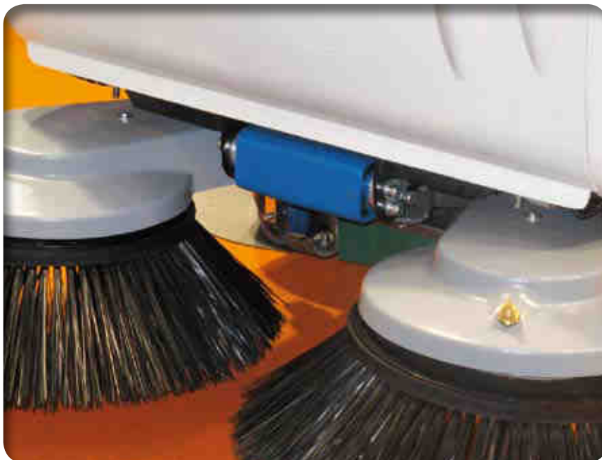
▲ Elastic suspension of rotary brush
