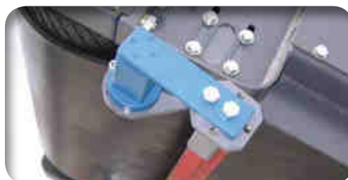
Elastic scraper suspensions for continuous belt cleaning
