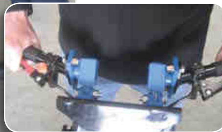
Resilient handle mounting for vibrating compactors
