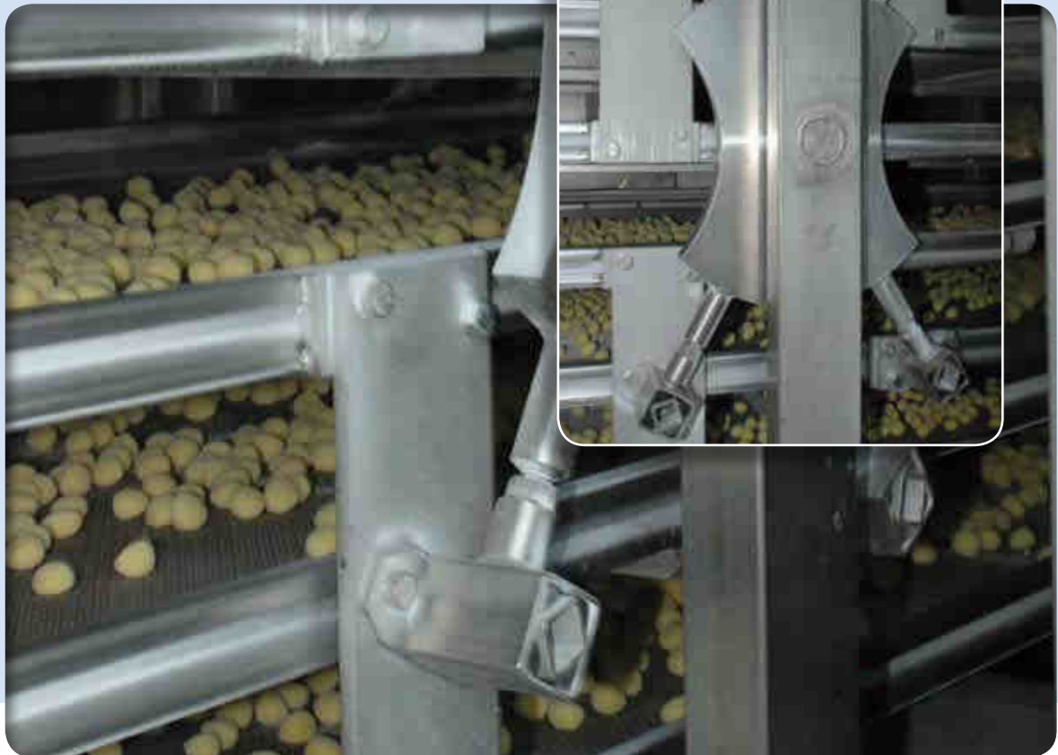
Heat resistant double rockers for pasta dryers
