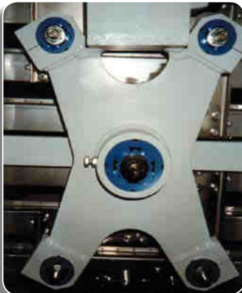
Heat resistant double rockers for pasta dryers
