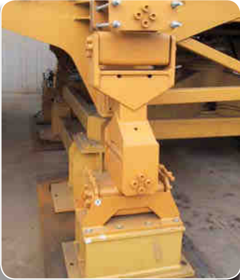
Universal joint suspensions for heavy duty chip-sorting sifter
