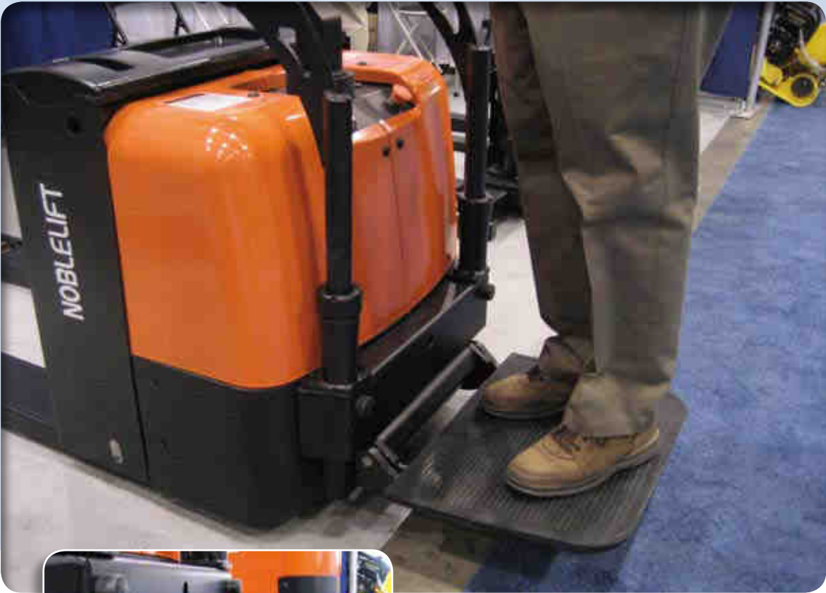
▲ Elastic suspension of driver platform on fork lifts
