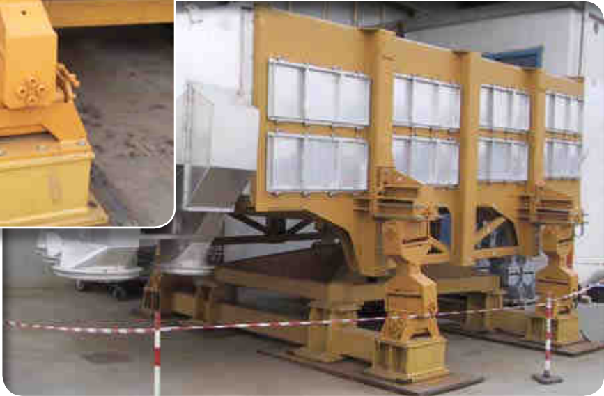
Universal joint suspensions for heavy duty chip-sorting sifter
