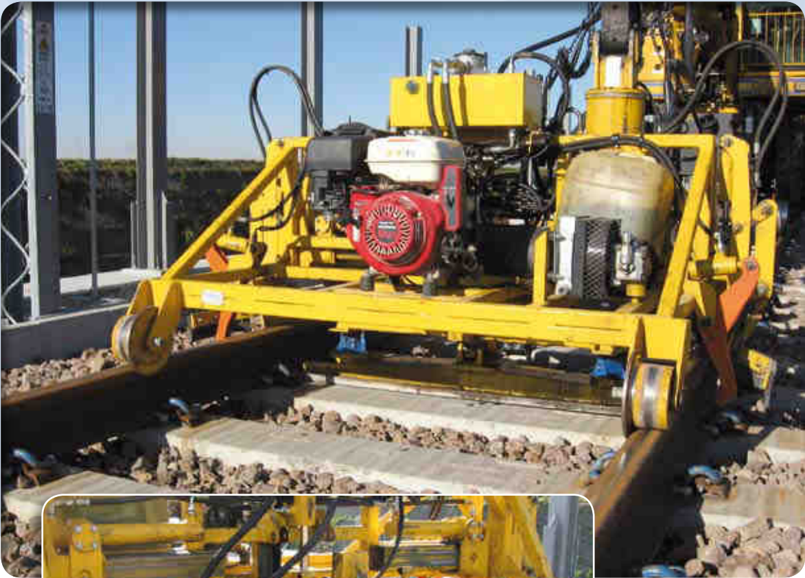
Cushioning suspension of railway-bed compactor
