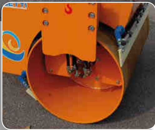
Elastic scraper suspensions for roll cleaning
