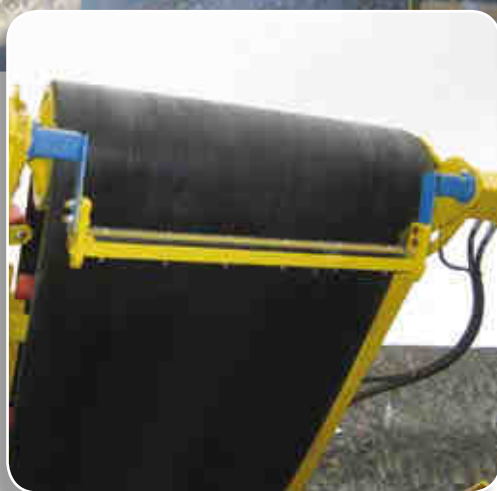
Elastic scraper suspensions for continuous belt cleaning
