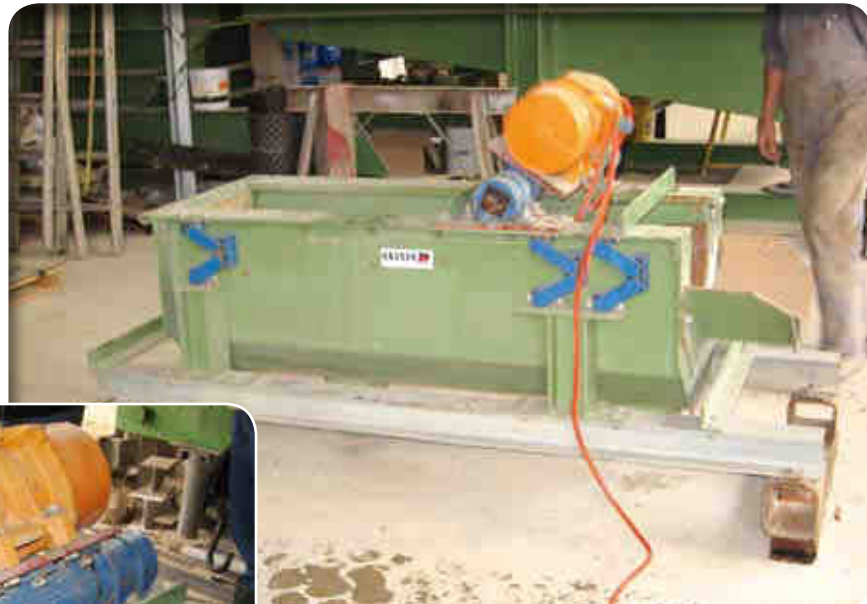
Elastic pendulum-suspension of single vibrators generating an ellipsoidal motion
