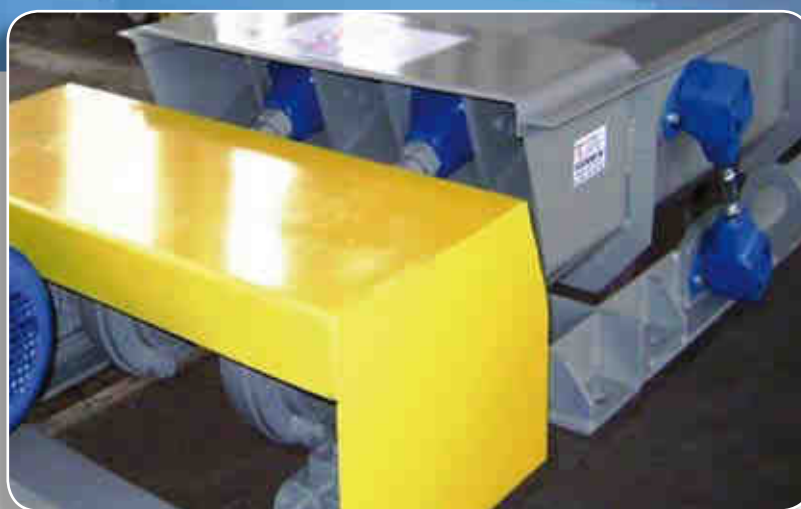
Elastic drive heads for crank driven troughs
