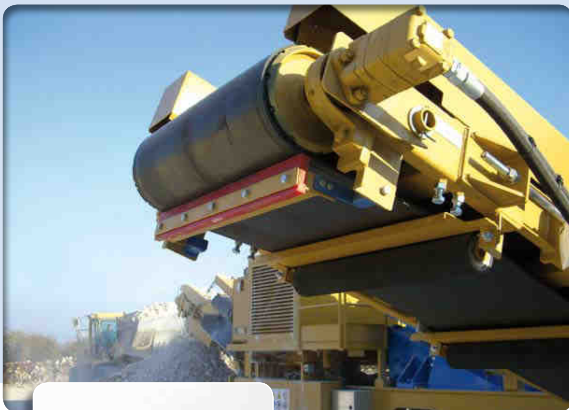
Elastic scraper suspensions for continuous belt cleaning
