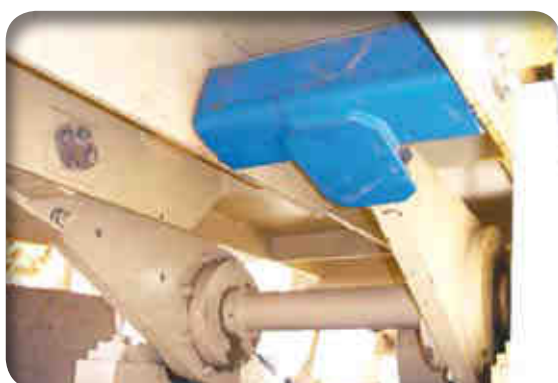
Elastic drive heads for crank driven troughs
