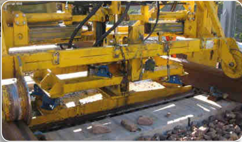
Cushioning suspension of railway-bed compactor
