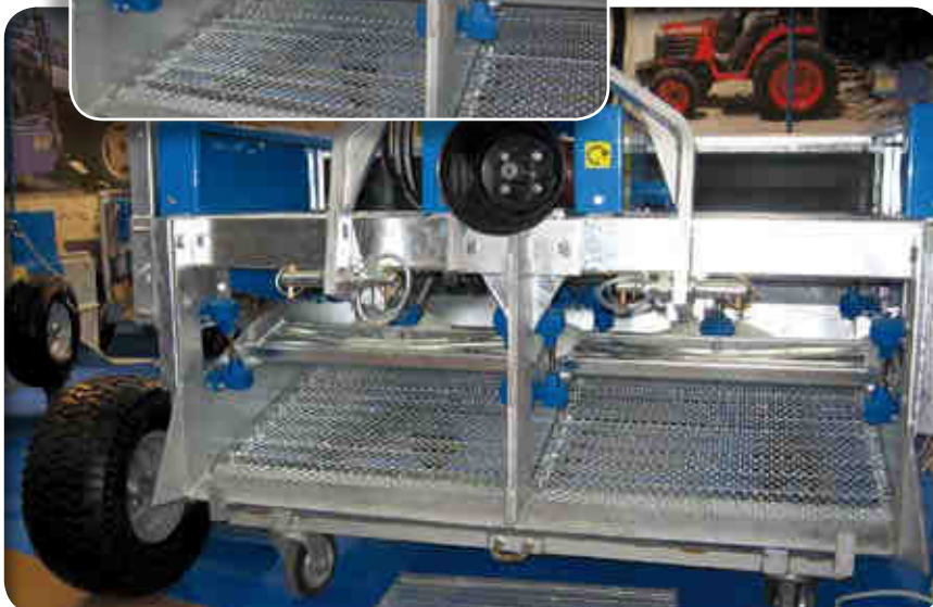
Elastic rocker suspensions for sand sifting screens
