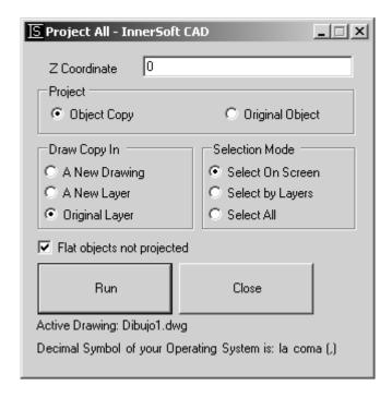
User must set a number as Z coordinate from menu. App will ask for an object's selection on AutoCAD screen. Every object in selection will be geometrical projected onto the X-Y plane at user input Z-Coordinate.
