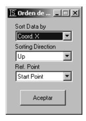
Once you press the OK button, this submenu closes and then the sorting conditions will apply to the selection that you get in AutoCAD.
