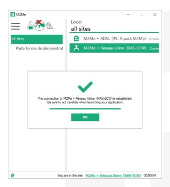
**Warning:** if you have specific SW to drive the maintenance of your PLC (PL7, Unity, So Machine, STep 7, TIA Portal, ...), please note that this SW must be on the PC equipped with the M2Me Client.
