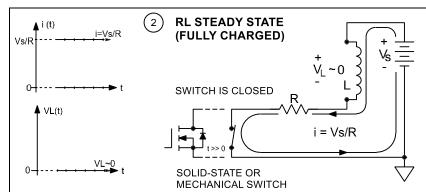
After charging, the inductor acts like a SHORT circuit to DC with i=Vs/R and VL $\sim$ 0. The potential energy stored in the inductor is w=0.5\*L\*(i)^2
