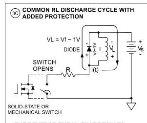
THE REVERSE EMF VL THAT RESULTS WHEN NORMAL CURRENT FLOW IS INTERRUPTED IN THE INDUCTOR IS CLAMPED TO A SAFE VOLTAGE LEVEL EQUAL TO THE FORWARD VOLTAGE DROP OF THE DIODE, PREVENTING IT FROM BEING DISTRIBUTED ACROSS THE WIRING BETWEEN THE SWITCH AND LOAD WHERE IT COULD RAISE EMISSIONS, DAMAGE THE SWITCH, AND WREAK HAVOC IN ADJACENT WIRING AND COMPONENTS.
