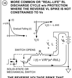
THE REVERSE VOLTAGE SPIKE THAT RESULTS WHEN NORMAL CURRENT FLOW IS INTERRUPTED IN THE INDUCTOR IS DISTRIBUTED ACROSS THE WIRING BETWEEN THE SWITCH AND LOAD AND WILL INCREASE NOISE AND EMISSIONS. ITS AMPLITUDE IS LESS PREDICTABLE AND IT HAS THE POTENTIAL TO ARC OVER, AND POSSIBLY DAMAGE THE SWITCH AND ADJACENT COMPONENTS.
