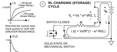
When the switch is closed, the inductor begins charging and initially acts like an OPEN circuit to DC and gradually becomes a SHORT circuit to DC. The current i rises from 0 to Vs/R, while the voltage drop in the inductor decreases from Vs to 0 (assuming an ideal coil resistance of 0 ohms).
