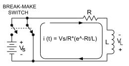
A VERY QUICK REVERSE VOLTAGE SPIKE, INITIALLY VL = -Vs, OCCURS WHEN NORMAL CURRENT FLOW IS INTERRUPTED IN THE INDUCTOR AND IT IS DISTRIBUTED ACROSS THE WIRING BETWEEN THE SWITCH AND LOAD. THIS TRANSIENT CAN COUPLE NOISE INTO ADJACENT WIRING AND COMPONENTS. AND BECAUSE IT IS APPLIED TO OUR SWITCH IN REVERSE, IT COULD DAMAGE THE SWITCH IF IT WAS A SOLID-STATE TYPE, LIKE A BIPOLAR JUNCTION TRANSISTOR.
