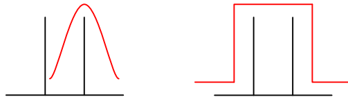
Figure 6: Two tone scenario, drawn with analog IF filters. Left hand side: narrow-band RBW filter, right hand side: wide-band image rejection filter.
