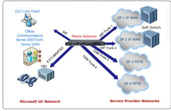
AudioCodes Media Gateways also offer simultaneous connectivity to several PSTN and SIP Trunking service providers, providing least cost routing and redundancy.
