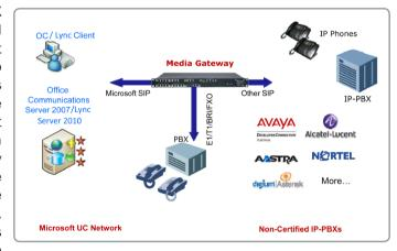
Communications Server / Lync Server is a lengthy process that can be reduced by using a Media Gateway that is already interoperable with both network components.
