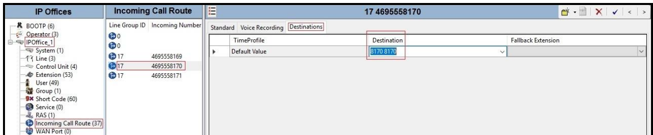
Figure 72 – Remote Worker Incoming Call Route
