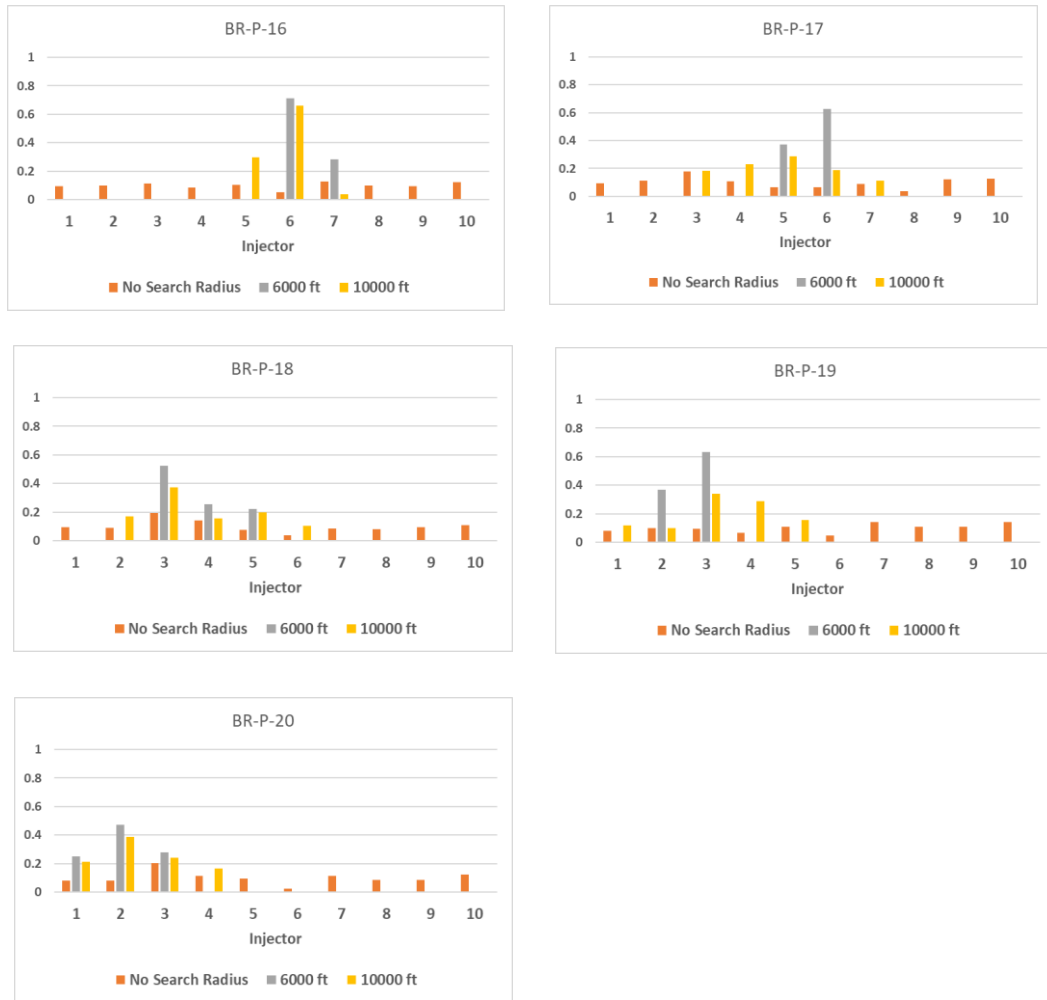
Figure 51 Normalized LSTM reservoir connectivity for: no search radius, 6000 ft, and 10000 ft (Well P16 – Well P20)
