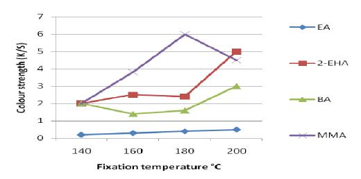
**Figure 3.** The effect of the type of binders used on the color strength of screen printed cotton fabrics using 3% Imperon Brilliant red B, the time of fixation is 2 min.
