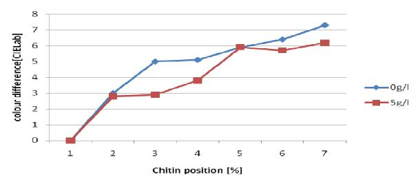
Figure 6. Changes in colour difference of polyester/ cotton fabric samples dyed using disperse/reactive Blue after chitin (II) NaOH concentrations 0 g/l and 5 g/l.
