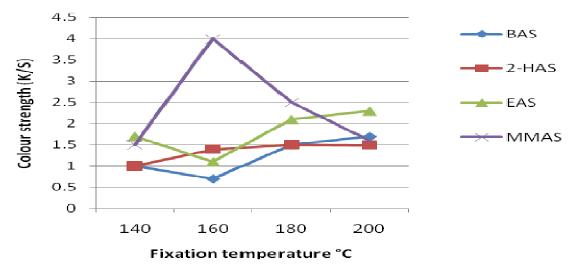
**Figure 4.** The effect of the type of binders used on the color strength of screen printed cotton fabrics using 3% Imperon Brilliant red B, the time of fixation is 2 min.
