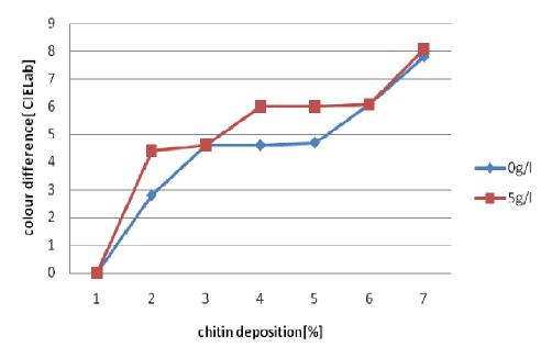
**Figure 5.** Changes in colour difference of polyester/cotton fabric samples dyed using disperse/reactive Blue after chitin (I) NaOH concentrations 0 g/l and 5 g/l.
