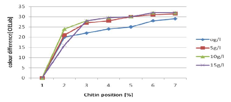
Figure 8. Changes in colour difference of polyester/ cotton fabric samples dyed using disperse/reactive Red after chitin (I) NaOH concentrations 0 g/l, 5 g/l, 10 g/l and 15 g/l.
