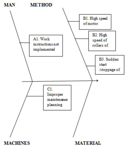
Fig-5: Fishbone Diagram for Dents
