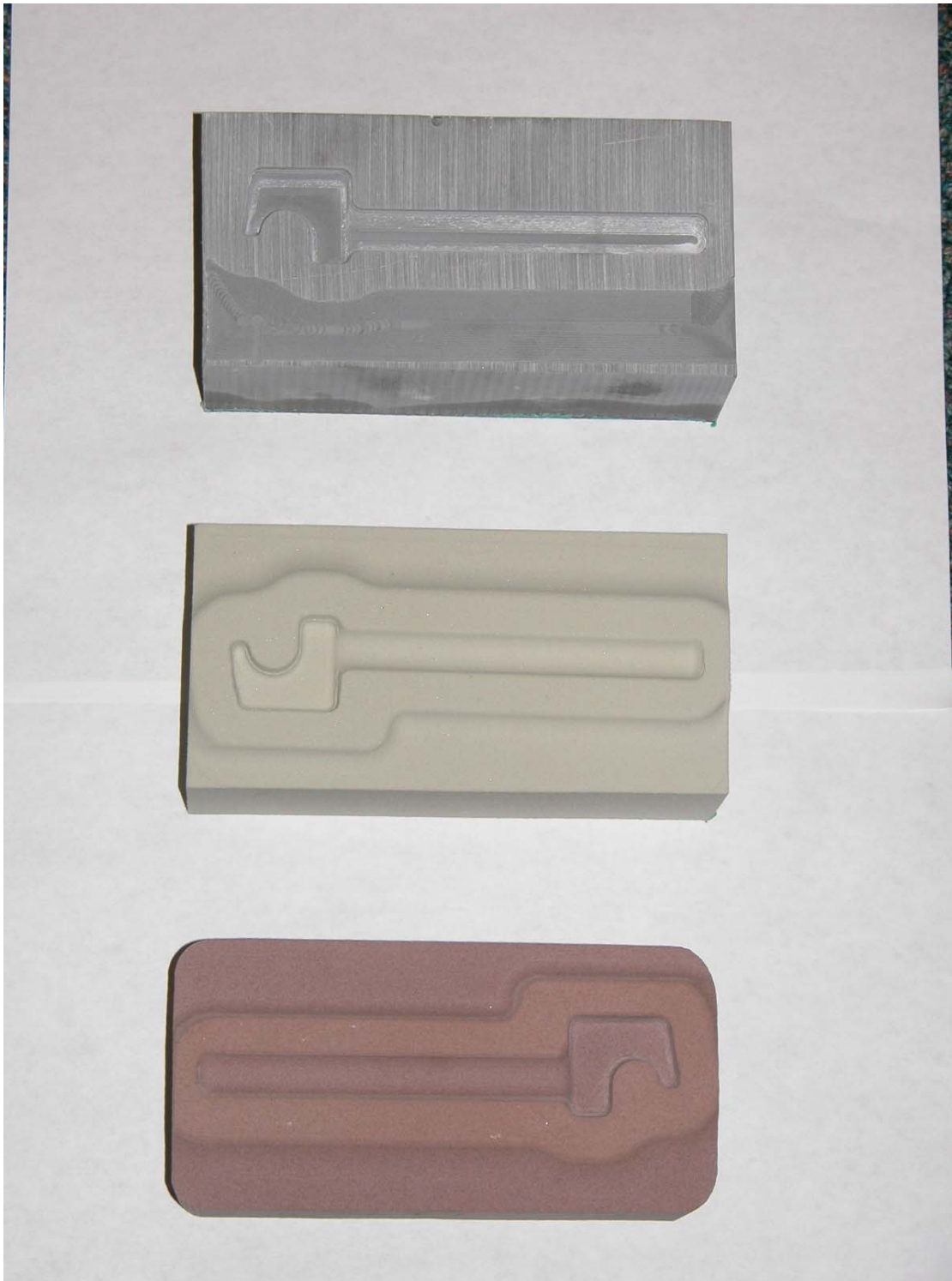
Figure 20: Different types of Ren Boards; A: Ren Board 5003,
