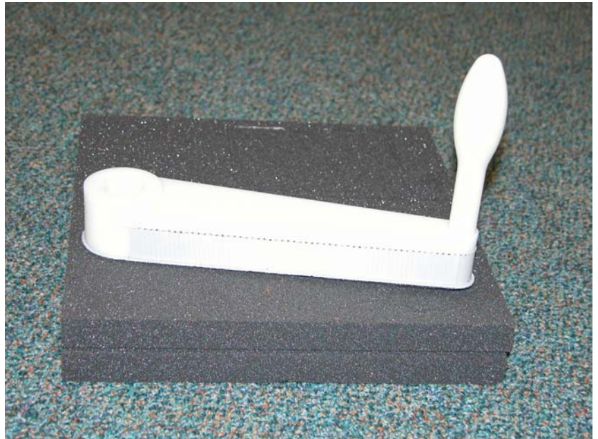
Figure 14: Hand Lever Produced by FDM
