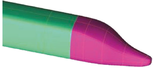
FIGURE 5: Bionic head type of high-speed trains based on hummingbirds.
