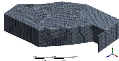
Figure 6.8 Tertiary Structure Initial Mesh for TO with 17117 SHELL181 elements
