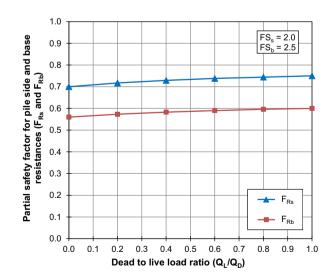
Fig. 6 Variation of  $Q_{\rm L}/Q_{\rm D}$  with  $F_{\rm Rb}$  and  $F_{\rm Rs}$  of the intersection point for SPT-based driven piles.
