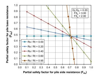
Fig. 7 Calibrated  $F_{Rs}$  and  $F_{Rb}$  with respect to the skin friction share for CPT-based driven piles.
