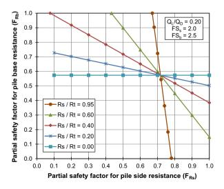
Fig. 5 Calibrated  $F_{Rs}$  and  $F_{Rb}$  with respect to the skin friction share for SPT-based driven piles.
