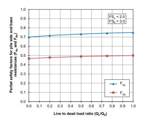
**Fig. 8** Variation of  $Q_L/Q_D$  with  $F_{Rb}$  and  $F_{Rs}$  of the characteristic intersection point for CPT-based driven piles.
