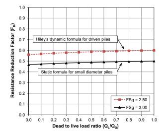
Fig. 3 Relation between calibrated  $F_{\rm R}$  and  $Q_{\rm L}/Q_{\rm D}$  ratio for static and dynamic formula design methods adopted in the ECP-202 (2001).
