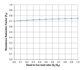
Fig. 4 Relation between  $F_{\rm R}$  and  $Q_{\rm L}/Q_{\rm D}$  ratio for the empirical load-settlement relationship design method of axially loaded large diameter bored pile and static pile load test design method at FS<sub>g</sub> equals 2.0.
