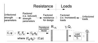
**Fig. 1** Schematic diagram for the concept of factored strength approach [9].
