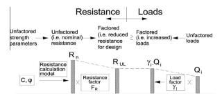
**Fig. 2** Schematic diagram for the concept of factored resistance approach [9].
