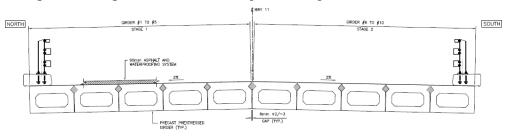
Figure 2. Typical MTO Adjacent Box Girder Bridge Deck Cross Section
