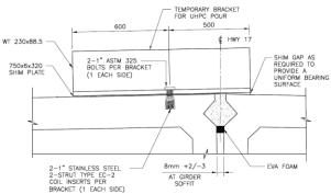
Figure 9. Temporary Centreline Joint Brace Detail
