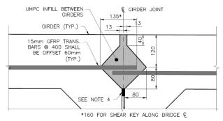
Figure 3. Typical Box Girder Longitudinal Joint Detail
