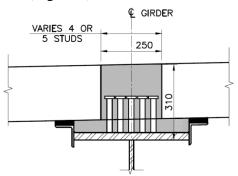
Figure 6. Typical Composite Connection Detail
