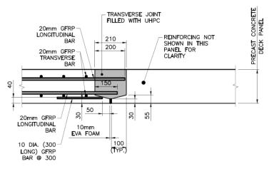
Figure 5. Typical Precast Deck Panel Joint Detail
