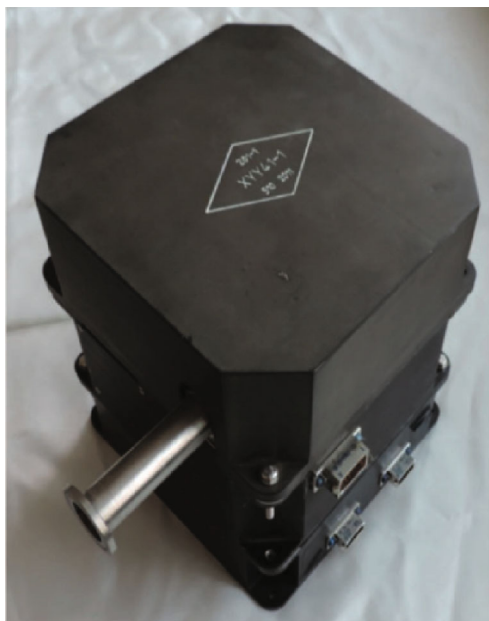
FIGURE 16: Miniature magnetic sector mass spectrometer developed in LIP [76].
