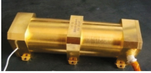
FIGURE 14: Physics package of rubidium atomic clocks developed in LIP.
