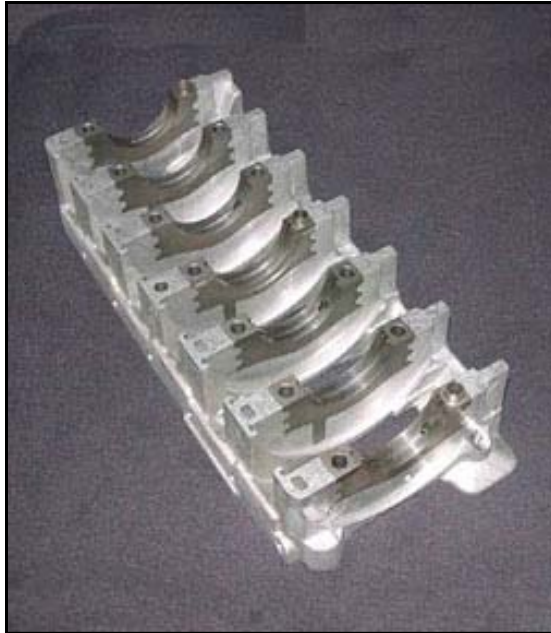
Ladder frame with casting grey iron bearings (high pressure die casting)
