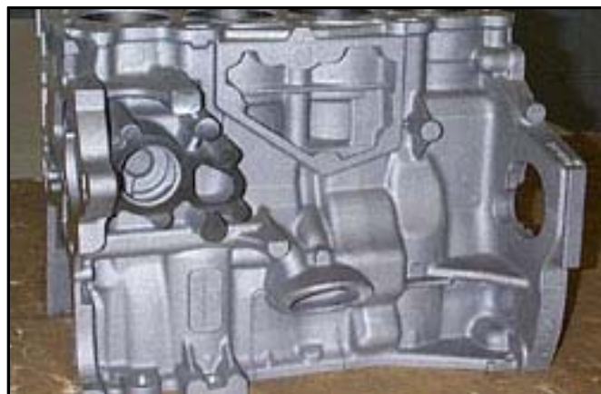
Side view of a Ford Zetec Block with pre-cast water pump housing and oil filter flange
