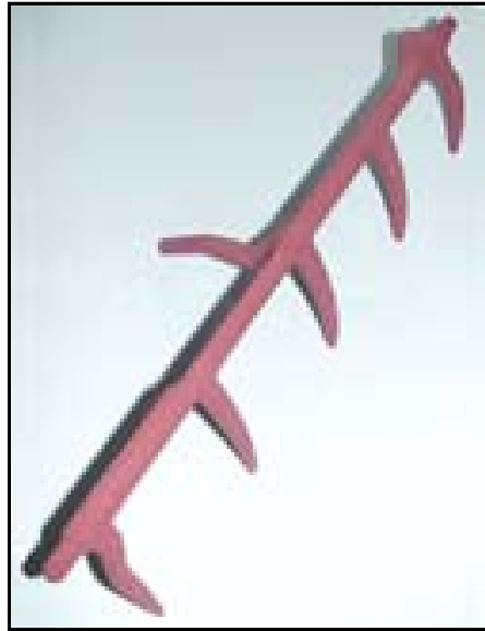
Oil gallery core for Ford Zetec 1.6L Block
