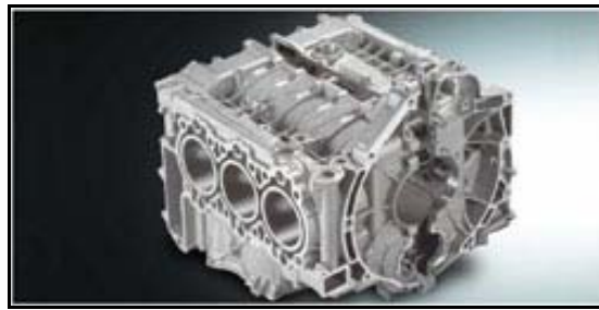
PORSCHE Boxter opposed-cylinder block halves with LOKASIL ® cylinder bore surfaces produced by squeeze casting
