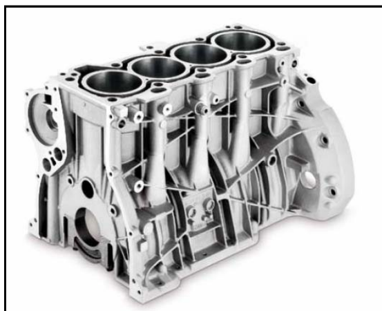
High pressure die cast deep skirt block of the Daimler A class in-line 4-cylinder engine with cast-in grey iron liners
