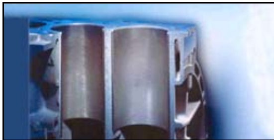
Ford Zetec Block with cast-in grey iron linings
