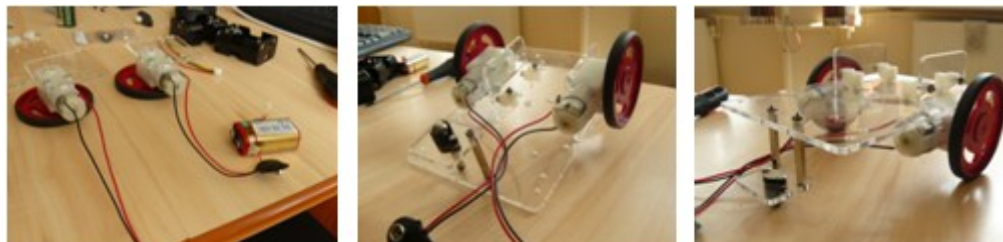
Figure 12. Securing the assembly wheels-motors on the chassis
