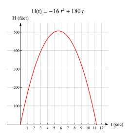
Note that the graph shows the height of the rocket H(t) as a function of time t. It does not show the path of the rocket. The rocket travels up and down along a vertical line.
