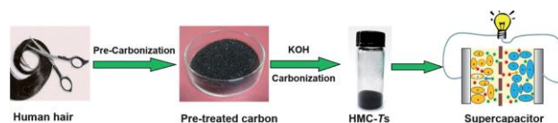
Scheme 4. Flow diagram for the fabrication of HMCs. Hair fibers are pre-carbonized at 300°C and then mixed with KOH (weight KOH : weight carbon \frac{1}{2} : 1) and further carbonized at 700, 800, and 900 °C, respectively.
